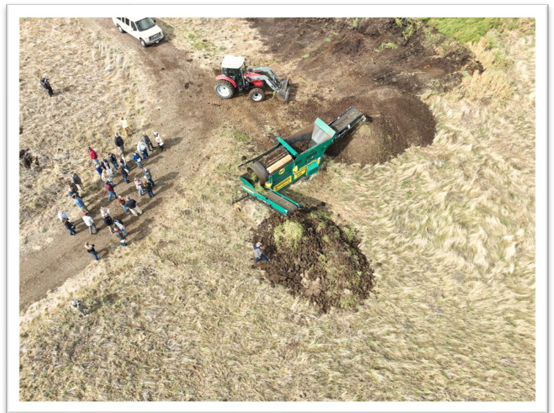
Trommel in use sorting through a manure pile
