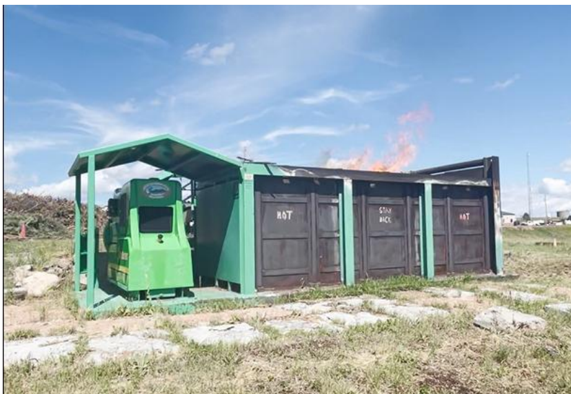
Air curtain burners can efficiently and safely consume fuels with less emissions than pile burning. Photo: The Ember Alliance.
