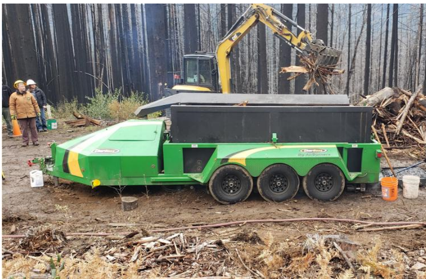
Biochar units can help mitigate wildland fuels and produce biochar that can improve soil health. Photo credit: U.S. Biochar Initiative.
